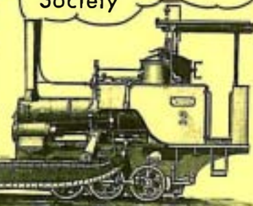
This remarkable double locomotive was the product of Charles Brown and featured a lever drive. It was built in 1878 at Brown's Winterthur factory for the narrow-gauge Villa Real and Villa Regoa tramway in Portugal. ( Recent Locomotives , Fig. 175)
