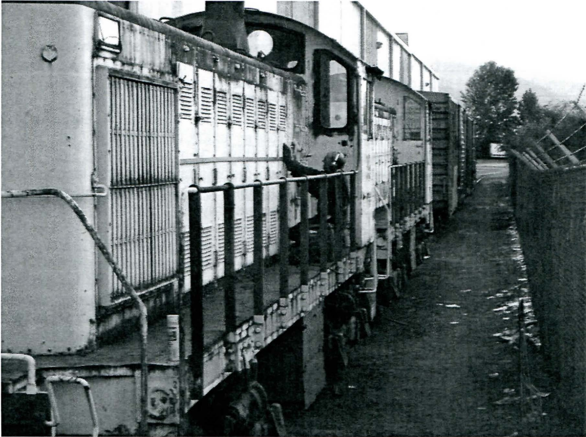
The Chapter's two S-2 locomotives with George Hickok welding a metal strip across the engine access doors.
