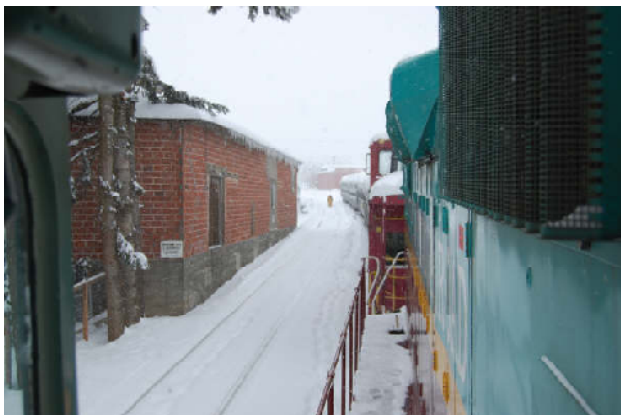
Above: The train made it to Parkdale, MP 21, but snow buildup prevented it from reaching the top of the line (Elev. 1740). There was too much snow to plow up the 3.6% grade with this train and the icing conditions. With all handbrakes applied, the train still slid downhill. (Photo by Leonard Morgan)
