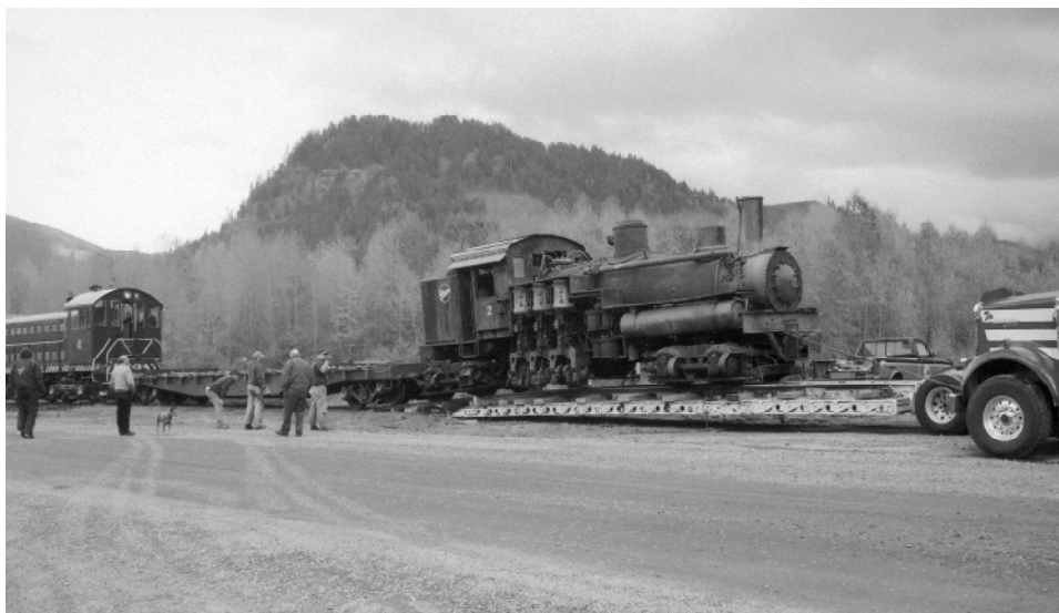
Hauling technology improved substantially in the years that the 2-spot was stored in Port Angeles. The 2002 move to Mount Rainier Scenic Railroad was handled quickly and efficiently. Here, a MRSR Alco eases the #2 from the trailer to its new home rails.
