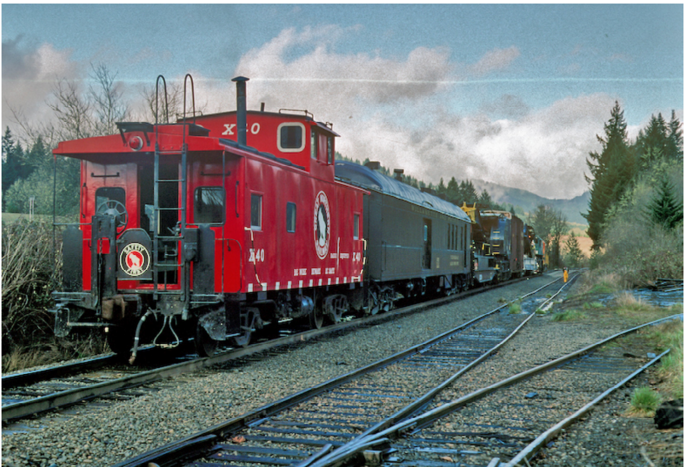
Opposite above: Portland and Western continuous-welded rail train on the Oregon Electric line dropping rail for the Morse Brothers Gravel Spur near Hopmere in 1995. Opposite below: Allan Carswell, former GN carman and Bruce's father, who helped restore X40. Photos from Bruce Carswell
