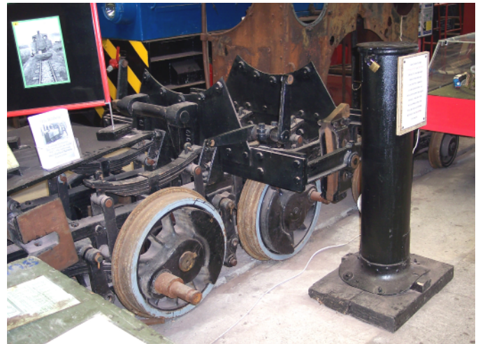
Left, above, and below: Scarcely more than a collection of parts, this Baldwin tank 4-6-0 now resides at the Welsh Highland Railway in Porthmadog. The locomotive was brought to Wales from India (#794) as an example of a Baldwin 4-6-0T (#590) that once operated on the Welsh Highland. A fund drive is underway to restore the locomotive to operating condition.
