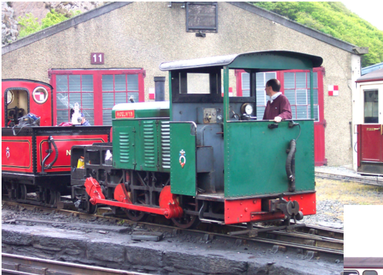
Left and below: The Moelwyn is a 1918 Baldwin product that now resides on the Ffestiniog Railway in Wales. The 2-foot gauge internal combustion locomotive was originally built for service in France. Her original prime mover has been replaced with a Gardner diesel and a lead truck added to make it a 2-B-0. Moelwyn is shown here performing shop switcher duties at Boston Lodge, about a mile from the main Ffestiniog Railway terminal at Porthmadog.
