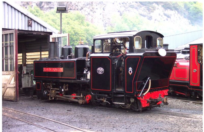
Left and below: The Mountaineer is an Alco Cooke 2-6-2T built in 1916. Originally constructed for the front lines of WWI as a trench locomotive, the Patterson, New Jersey product has seen much rebuilding in her nine-plus decades of service. The Mountaineer is currently out of service on the Ffestiniog Railway, awaiting boiler work. In the recent past, she had the distinction of hauling trains on the newly reopened sections of the Welsh Highland Railway.
