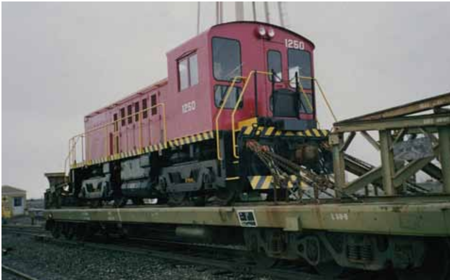
Locomotives were changed with reasonable frequency at the Umatilla Depot. These photos show RS-4-TC #1250 being readied for shipment on a heavy-duty flatcar.
