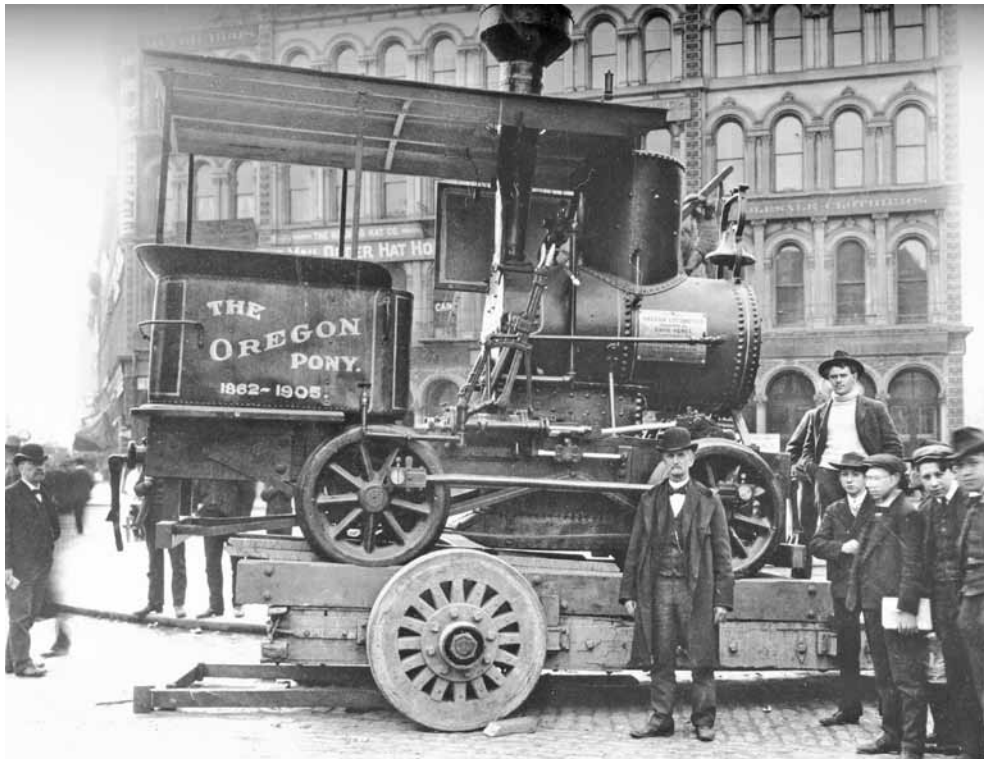
All duded-up for a stint on display at the 1905 Lewis and Clark Exposition in Portland, the Oregon Pony was given a two-gallon overhaul by its San Francisco owner, David Hewes. In 1904, the locomotive had fallen victim to a warehouse fire and lost both its wood parts and paint. The cosmetic restoration was respectable, and certainly preserved the important features of the locomotive. (Labbe collection, Oso Publishing, Timber Times )
