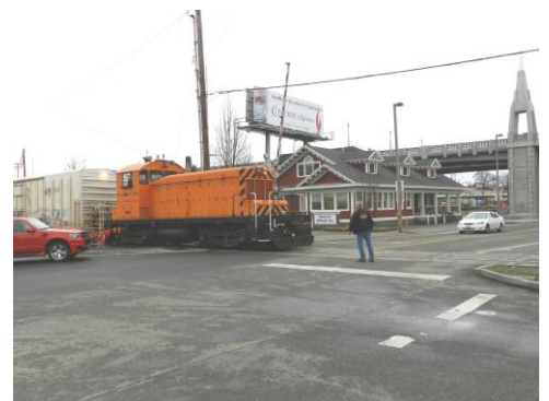
Portland Traction Company #100 Owned by the Oregon Pacific Railroad, 1952 EMD SW1, V-6 - 600 h.p. crossing near the existing Inman-Poulsen Building (Photo by Dave Larsen)
