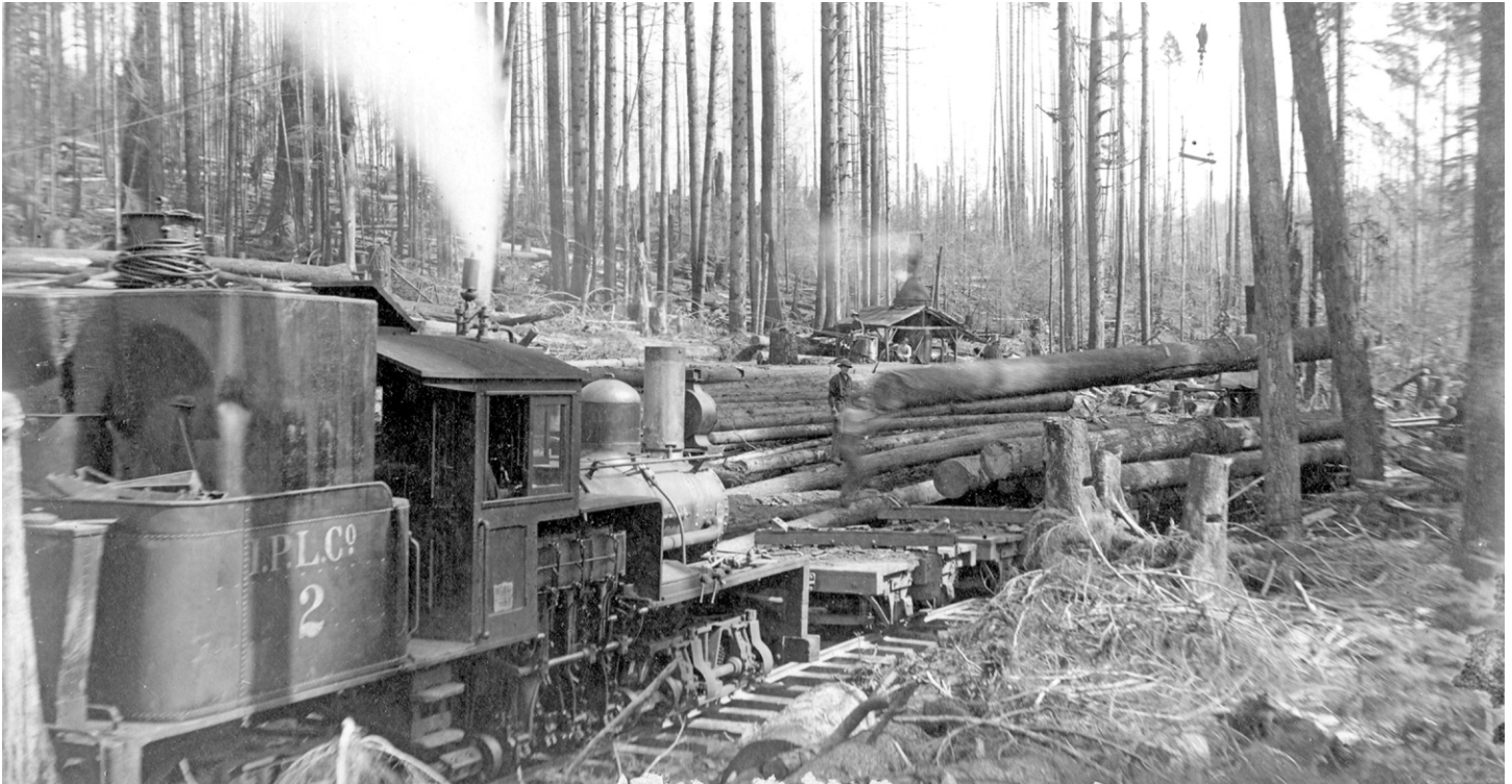
Inman Poulsen Lumber Company - Shay Locomotive #2 Loading Logs at Mt. Solo, WA (Collection of Camp 18, Gordon Smith)
