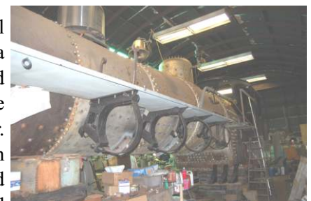
The running boards are installed and the hangers for the air reservoirs can be seen on this right forward view of the locomotive.
