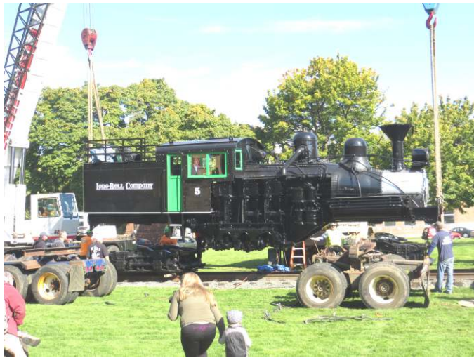
The Shay being lifted onto its Trucks
