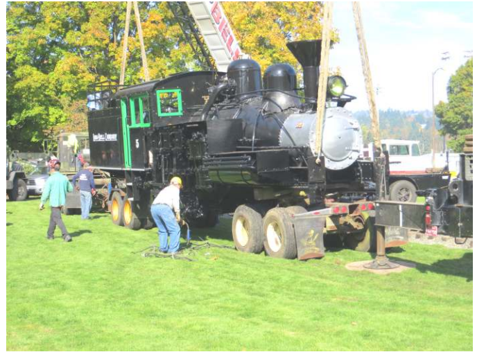
The Shay being lifted off of its temporary wheels
