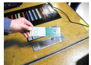
RFID Tag used for Automatic Equipment Identification (AEI)
