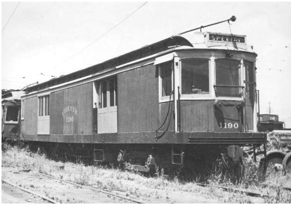
This view of 1190 from the 1940's shows the car after it was converted to a fire car. A reservoir filled most of the body and new pumps were installed. The car was also used for weed spraying (Jerry Risberg photo)
