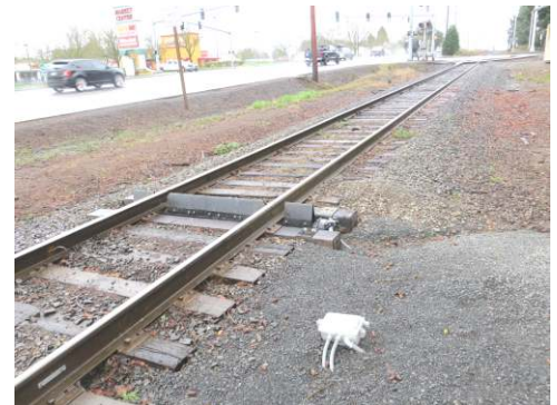
New Defect Detector on the Portland & Western
