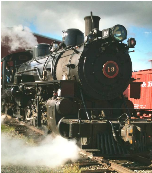
A recent photo of Sumpter Valley No. 19, a type 2-8-2 steam locomotive built in 1920, which was restored to operating condition in 1996, Photo provided by Alfred Mullet
