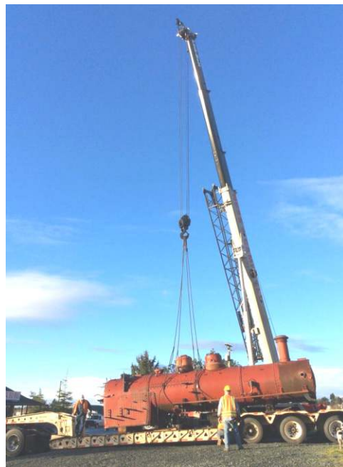
Lifting the Boiler onto the trailer for transport
