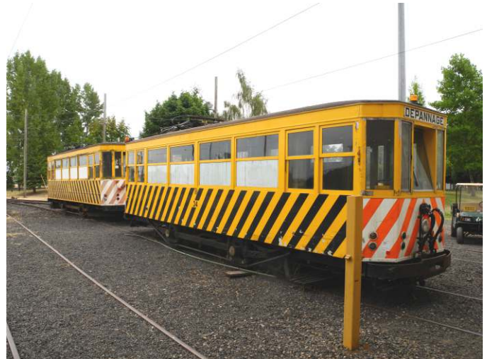
No. 19 (Left) "works" car is double ended. It is a converted passenger tram that became a sweeper car. It has brushes located under the car to sweep dirt and light snow off the trolley right-of-way. The car was originally built in 1934 as car No. 1052. It was converted by STIB into a work car No. 38 in 1970, then converted again in 1981 to No. 19. No. 34 (Right) was built by Le Tramways Bruxellois in 1934 as car No. 1290. It was converted to work service in 1971 and renumbered as car No. 34.
