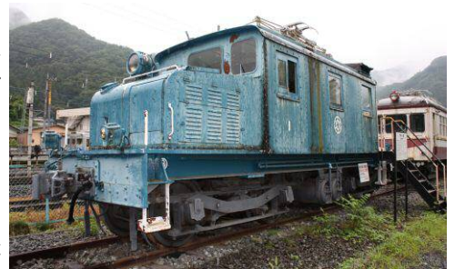
Electric locomotive Deki-1 was built by Baldwin-Westinghouse in 1922 as part of a five unit order by the Chichibu Railway. As originally constructed, the locomotives were supplied with 600VDC at the wire. In 1952 the railway changed its voltage to 1500VDC.
