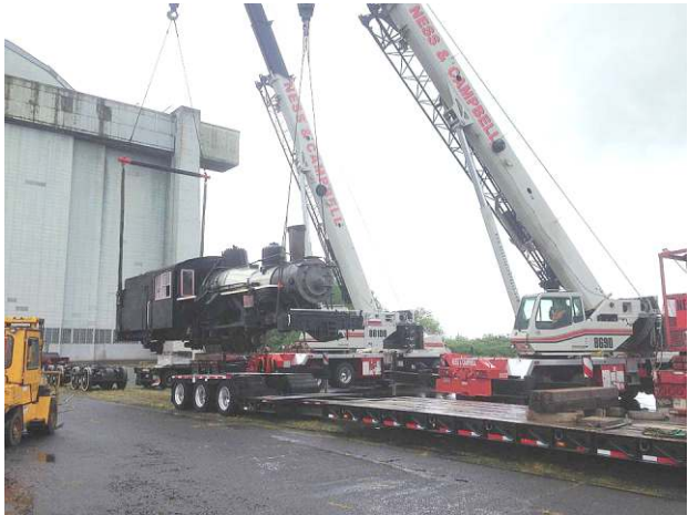
Being Lifted from the Transport Trailer
