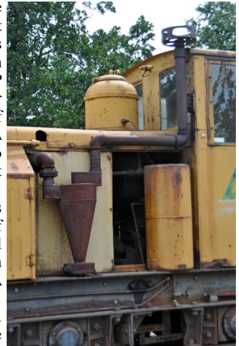
A cyclone separating spark arrester on the Plymouth No. 4
