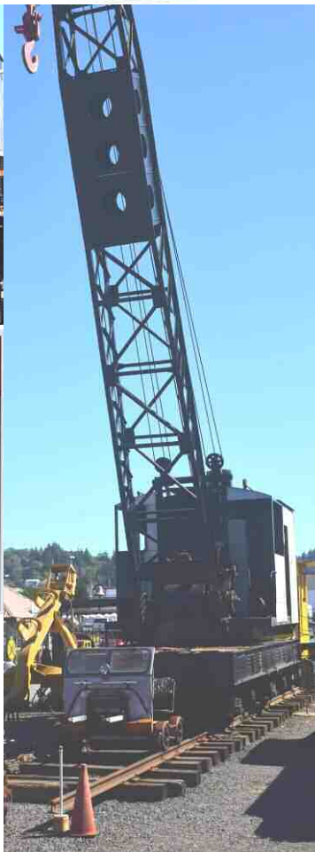
This 25 Ton Steam Powered Crane was built in 1927 by the Ohio Locomotive Crane Company. This crane was used by the George H. Chaney Logging Co. in and around Coquille from 1927 to 1933. It later worked for the Tacoma Belt Line Railroad.
