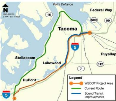
Passenger trains, including Amtrak Cascades, must slow down due to curves and single-track tunnels on the BNSF Railway main line tracks (green line) near Point Defiance and along southern Puget Sound. This project will reroute passenger trains to a bypass rail line along I-5 (orange line).
