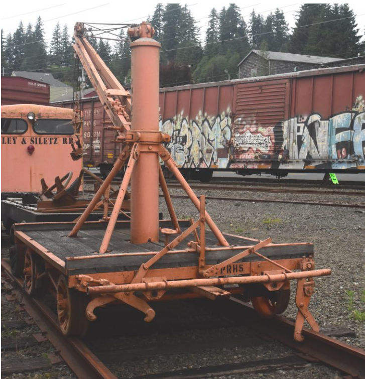
Bill Bain noted this unique mechanism on the small speeder crane during my recent visit to the Yaquina Pacific Railroad Historical Society in Toledo, Oregon. I was fascinated by the lever which moves the clamps to hold it to the rail, as shown in the lower right of the photo. (Text and Photo by T. Trent Stetz)
