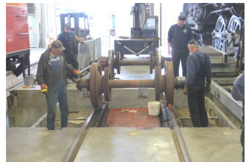
New Wheelset Rolled onto Table
