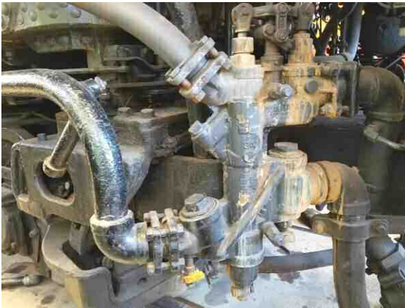
Photo of SP&S No. 70 Steam Injector, Located below the Fireman's side of the Cab
